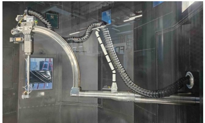
Fig. 18. C-strut test rig injected into the test section. The large black tube is the cable management system.
