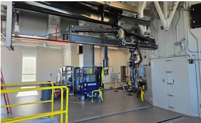
Fig. 17. Overhead-rail mounted RBS test rig in the retracted position. The deployable work platform is at left with yellow safety rails.
