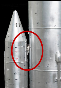
Transonic buffet environment due to booster forward attachment protuberance
