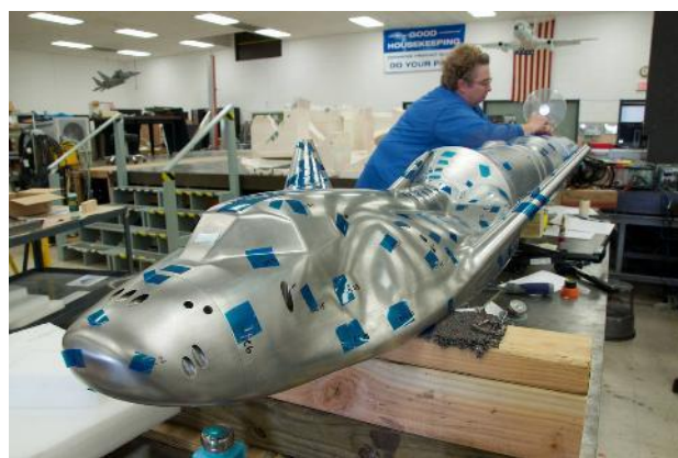
Integrated Wind Tunnel Model: Crewed Dream Chaser on Atlas V 2014
