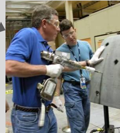
RCC panel drill tests
