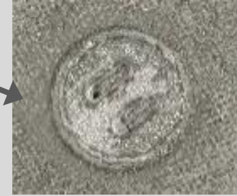
Fastener post arc jet test
